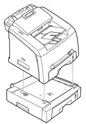
**5** Plug the interface cable of the tray into the optional tray connector on the back of the machine.
